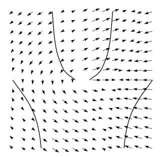
Fig. 3. Vector-field m for the half-integer dislocation combined with the semi-vortex of the magnetization. Solid lines indicate constant DW phases. Due to the presence of the half-integer dislocation, the number of sites changes between the upper and the lower rows from 2.5 periods (6 + 6 + 3) to 2 periods (7 + 5)
