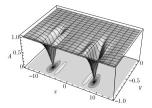
Fig. 2. A static array of dislocations appearing in the electric field applied transversely to the direction x of DW displacements
