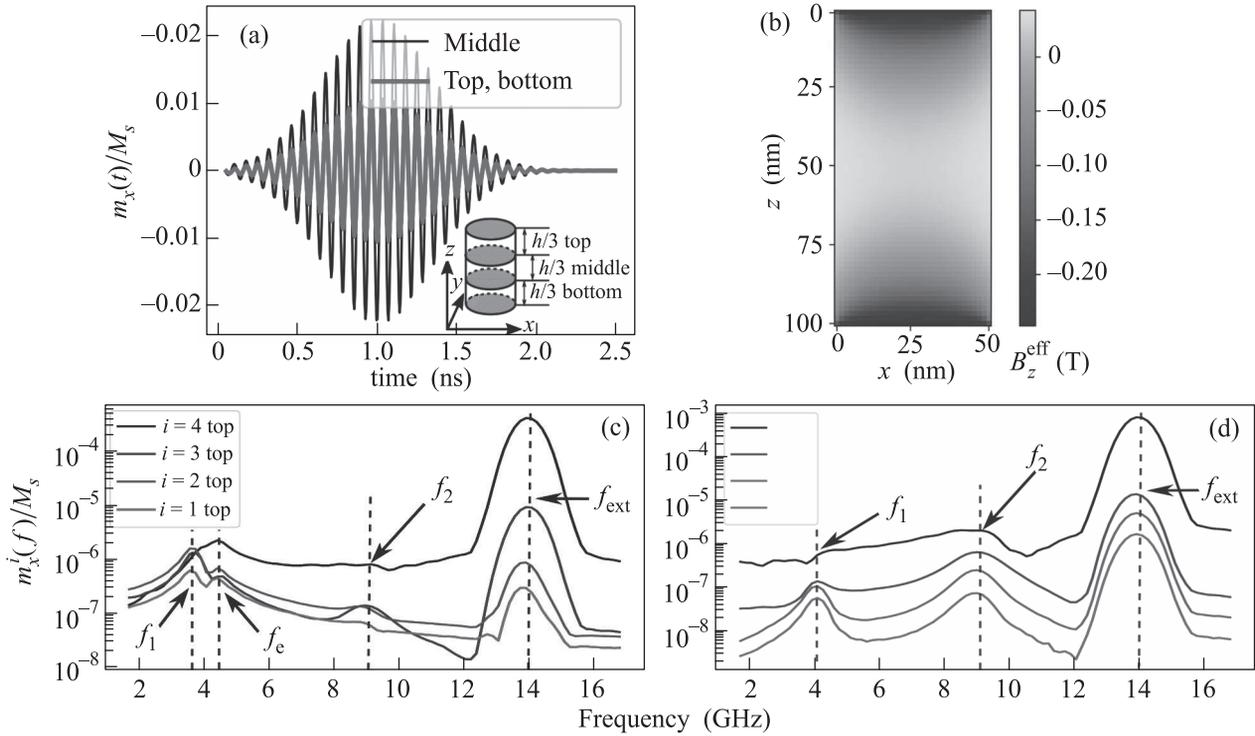
Fig. 1. (Color online) (a) – The amplitude of magnetization oscillation  $m_x(t)/M_s$  averaged over the different regions of the pillars. (b) – The distribution of the effective magnetic field  $B_z^{\text{eff}}$  inside the pillar. Magnetization amplitudes  $m_x^i(f)/M_s$  distribution in the frequency range  $f$  for the linear chain of  $N = 7$  pillars with numbers  $i = 1, \dots, 4$ , where magnetization is averaged over the top (c) and middle (d) regions of each pillar
