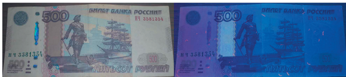
Fig. 4. Images of the same banknote under visible (left) and ultraviolet (right) illumination, where a bright fluorescent area stands out.
