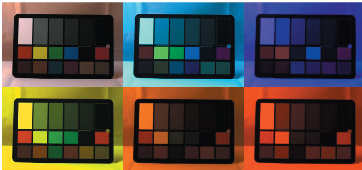
Fig. 3. Images of the same color table taken with the Canon 5D Mark III camera with fixed settings, but under different illumination conditions. This visually demonstrates the color metamerism phenomenon: the colors in different areas of the color table match or differ depending on the lighting. The images are reproduced from the MLSDCR (Multiple Light Source Dataset for Colour Research) (Smagina et al., 2020).
