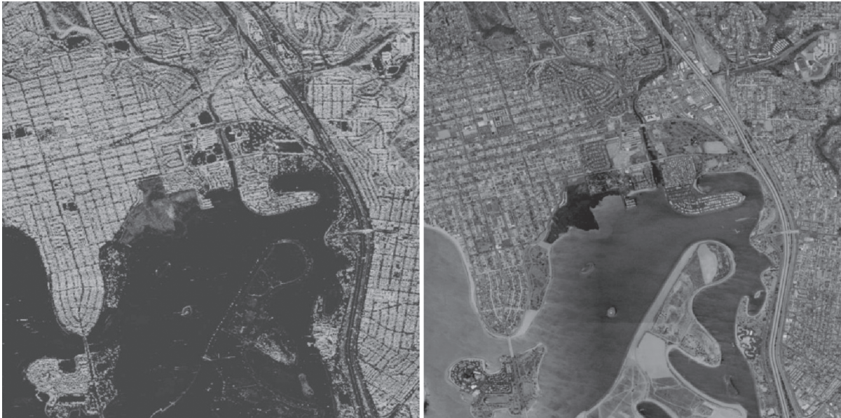
Fig. 1. Images of the same area of the Earth surface taken in the radio (left) and optical (right) spectral bands. The images are reproduced from (Abulkhanov et al., 2018).
