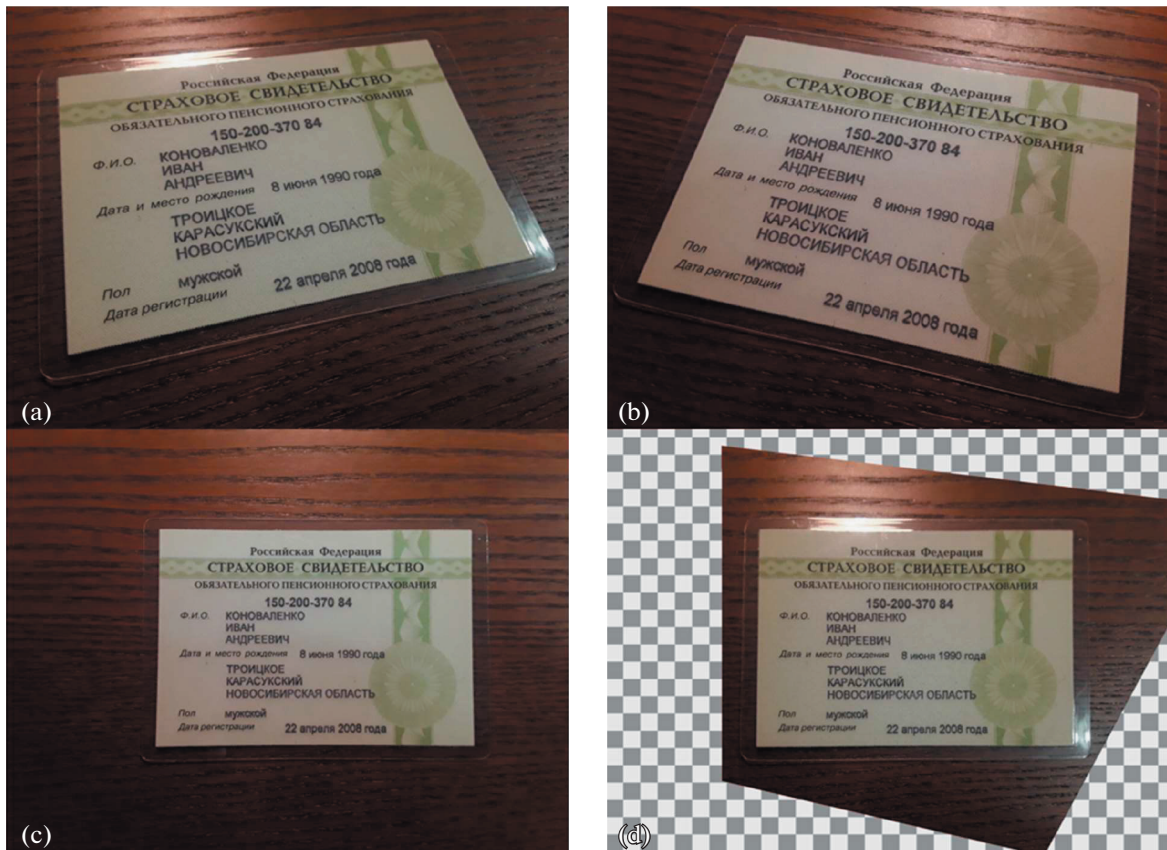
Fig. 5. Images of the same document. Images (a), (b), and (c) are captured from different angles. Image (d) is the result of geometric normalization of image (b) assuming that the capturing angle of image (c) is chosen as the normal imaging condition.
