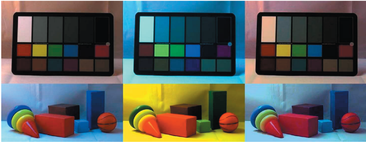
Fig. 16. Projective color normalization. The left images were obtained under the illumination chosen as normal, the center images were obtained under some other types of illumination. On the right, the results of projective color normalization of the central images are shown.
