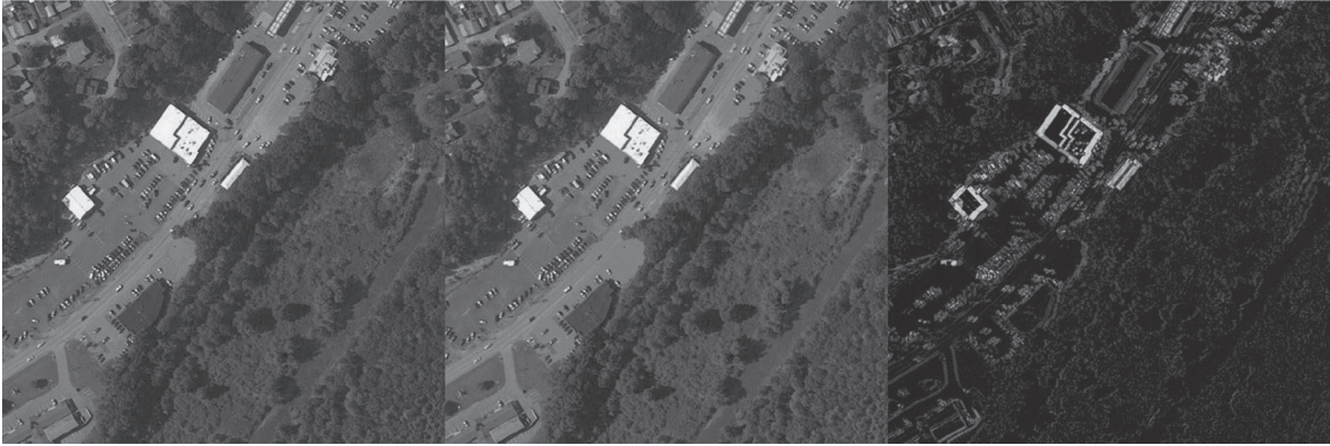
Fig. 9. Single-channel images I_{\text{ideal}} , I_{\text{alg}} and their difference module |I_{\text{alg}} - I_{\text{ideal}}| . The images are reproduced from (Goshin et al., 2014).
